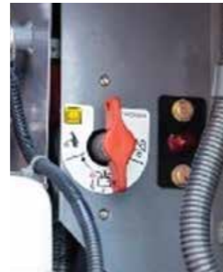
Disconnect Switch (Standard)
