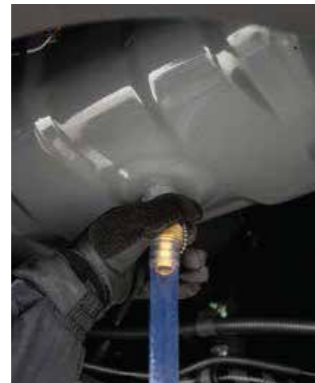
Simplified drainage of engine oil (Standard)
