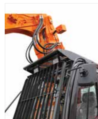
OPT Level II guard with opening / closing function (Standard)
