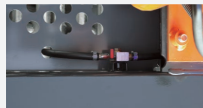
Fuel tank water drainage cock
