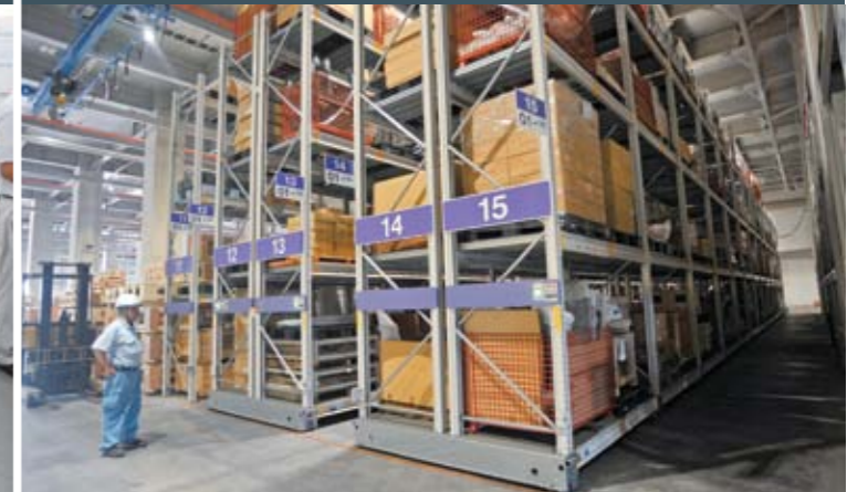
Large, electric movable racks make best use of space. Workers can move shelves and also store or take out parts from the top in one switch.
