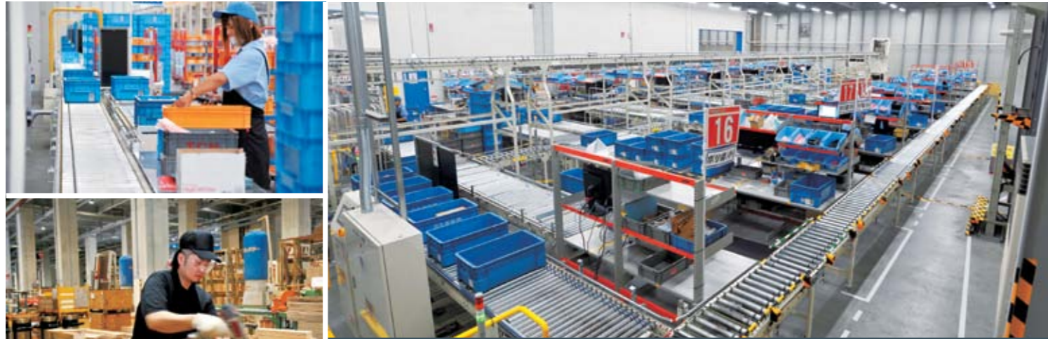
Small parts bearing information such as name, quantity, weight and date that are translated into bar codes are kept in a fixed location. Automatic input of data and reading improves efficiency. The ordered parts in each blue box are separated on the conveyor belt automatically.
