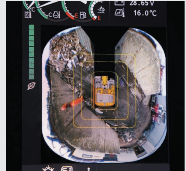
AERIAL ANGLE (Optional) 270-degree bird's eye-view camera system is available as an option.
