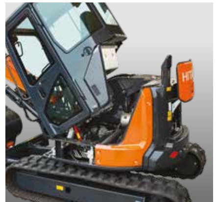
The tilting floor enables easy access to the engine and control valve for quick servicing.
