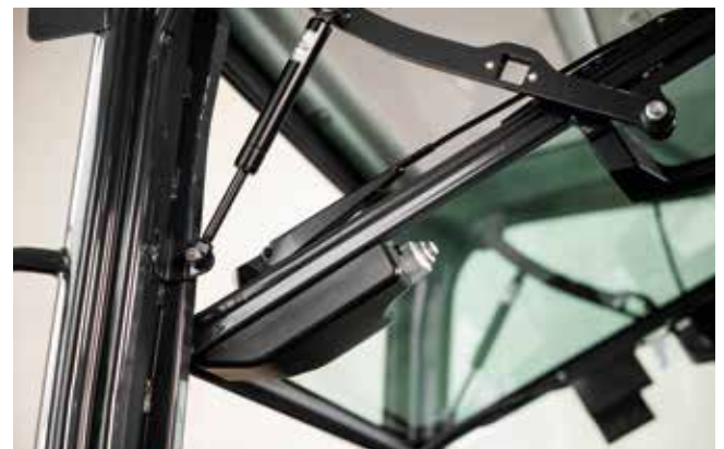
Power-assist front window opens smoothly and easily.
