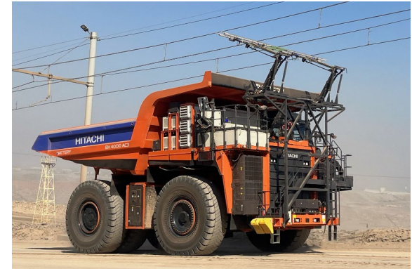
Full battery rigid dump truck with trolley
