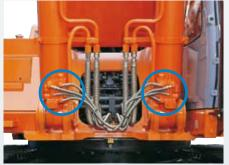
Due to hydraulic oil retention rapid lowering of the boom is prevented even in the event of boom cylinder hose rupture.
