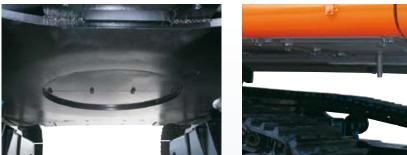
Protect the covered hoses, piping and valves from damage by collision with obstacles (reinforcements, etc.) during operation.
