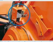
Alerts the operator of excess lowering angle of the boom of the high reach demolition front by sounding buzzer.
