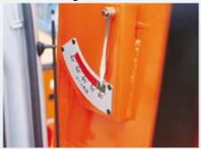
Indicates the high reach demolition arm inclination angle.
