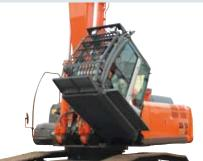
The cab can be tilted up to 30° for effortless elevated operations, without need for looking upward, reducing operator's fatigue.
