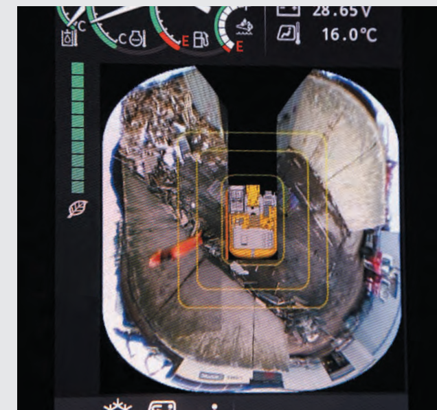
AERIAL ANGLE (Optional) 270-degree bird's eye-view camera system is available as an option.
