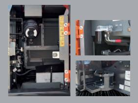
• The boarding platform adopts a D-section frame which improves overall strength against external impact. • The X-beam of the undercarriage adopts a reinforced welded structure where the upper and lower plates
