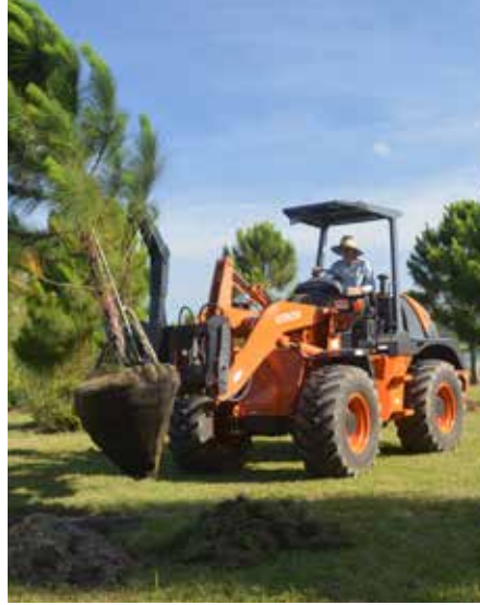
Outfitting Hitachi wheel loaders with a tree boom allows Springer to fine tune placement with minimal turf disturbance.
