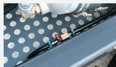
Fuel tank water drainage cock
