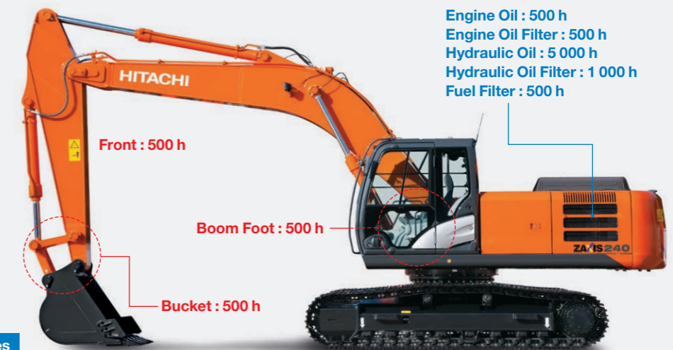
Note: Periodic inspection is required to check oil contamination and likes.
