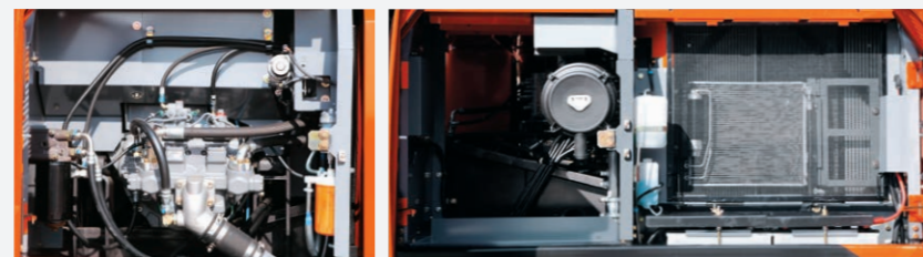
Grouped remote filters and inspection points
