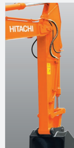
Attachment basic piping
