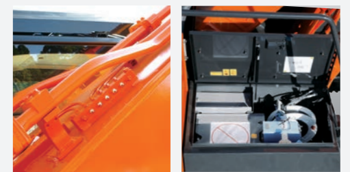
Centralized boom and arm greasing points Electric grease gun with hose-reel (Optional)
